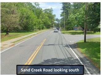
The southbound and northbound approaches on Sand Creek Road consist of one 11-foot lane in either direction. The Mordella Road approach is stop-controlled and consists of a single 11-foot shared left/right turn lane. Mordella Road is frequently utilized by residents and commuters as a connection to Central Avenue. There are no marked crosswalks at the intersection.
