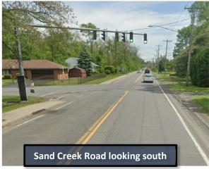
The southbound and northbound approaches on Sand Creek Road consist of one 11-foot lane in either direction. The Sunset Boulevard approach consists of a single 11-foot shared turn left/right lane. There is a marked crosswalk in poor condition along the Sunset Boulevard approach.
