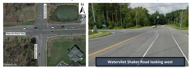
Currently there is a construction project that is underway along Watervliet Shaker Road that includes the intersection of Watervliet Shaker and Sand Creek Road. The work at the intersection consists of traffic signal improvements, additional travel lanes, ending a multi-use path at the southwest corner of the intersection and pavement rehabilitation. The limits of work for this project end along Sand Creek Road end at the south most driveway entrance to the Community Reformed Church of Colonie.
