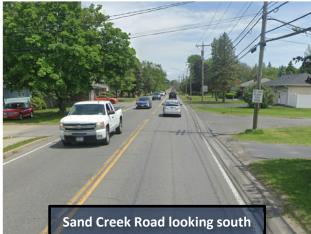
The southbound and northbound approaches on Sand Creek Road consist of one 11-foot lane in either direction. The Space Boulevard approach is stop-controlled and consists of a single 11-foot shared left/right turn lane. There are no marked crosswalks at the intersection.
