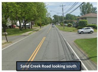
The southbound and northbound approaches on Sand Creek Road consist of one 11-foot lane in either direction. The Peter Drive approach is stop-controlled and consists of a single 12-foot shared left/right turn lane. There are no marked crosswalks at the intersection.
