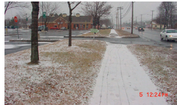
In front of new developments a landscaped buffer (tree lawn) should be provided between the edge of the curb and sidewalk.
